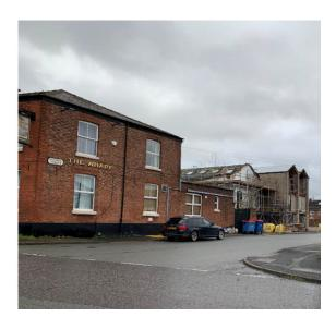
This building is too low to provide the necessary coverage to the target coverage area. It also has a hipped roof which is unsuitable for a telecommunications installation. There is insufficient space in the yard area to accommodate a radio base station at this location. A site at this location has therefore been discounted.
