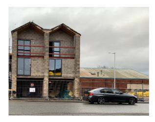
This is a single storey unit behind the application site. The construction materials of this building would not support a telecommunications installation. The building is also too low to provide the necessary coverage to the target coverage area and the roof is pitched and would not support a telecommunications installation. This site has therefore been discounted for these reasons.
