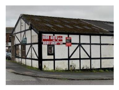
This single storey building is too low to provide the necessary coverage to the target coverage area. It also has a pitched roof which is unsuitable to support a telecommunications installation. The roof also contains skylights which prevent an installation from being built. It is of fragile construction in any event and would not support the weight of the telecommunications equipment.
